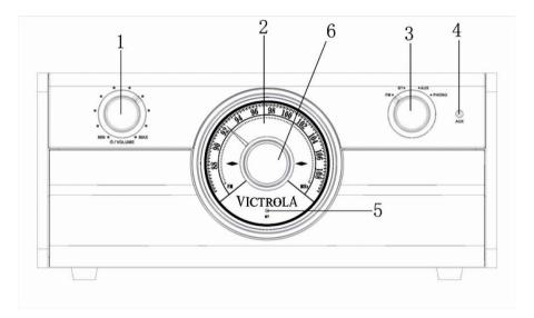
**POWER** O/**VOLUME**: Rotate clockwise to turn the unit ON. 1.
