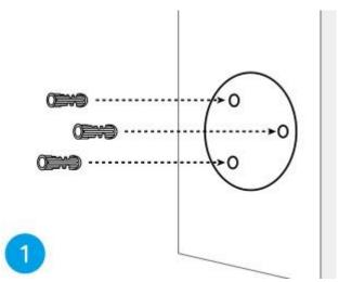
**Step 2.** Install the mount base with the mounting screws included in the package. (For WiFi cameras, please install antenna in advance)
