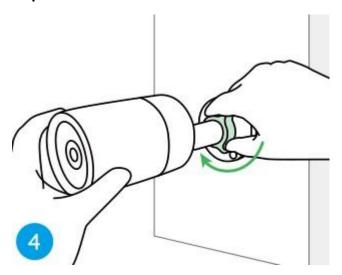
**Note:** If your camera has another mount without the adjusting knob, please loosen the adjusting screw with the provided hex key and turn the camera as shown below to adjust the angle.
