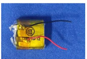
Lithium ion Battery Charging Case 761435 Golden CEL 3.7V, 350mAh, 1.3Wh
